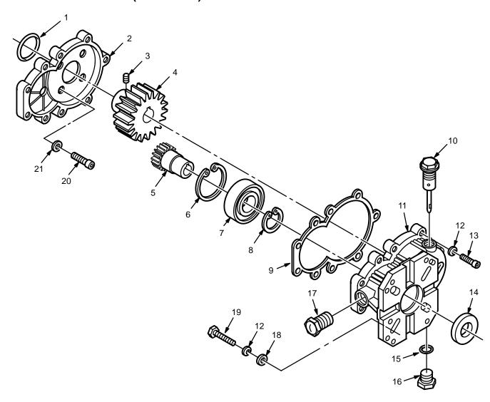
PARTS LIST 802-143 Gear Reducer (Model 2040)
